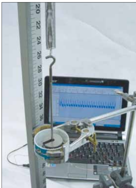
Figure 1. The experimental set-up used to analyse the timing of a mass–spring oscillator. The magnet (not visible) is located under the hanger.
