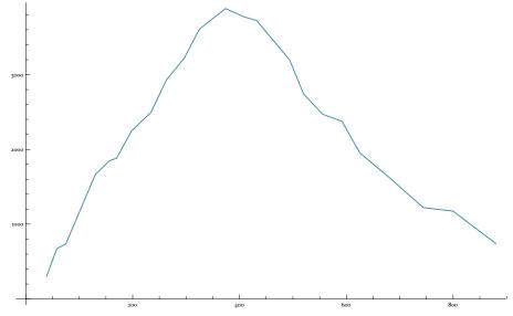
The retention function for the whole body of Cs-137 (that is for an acute intake "1" in t=0) is  $qWbCs137[t1_] = qWholebody[compartMatrix[caesium], 1, 1, t1, Log[2] / (30 * 365.24)]$
